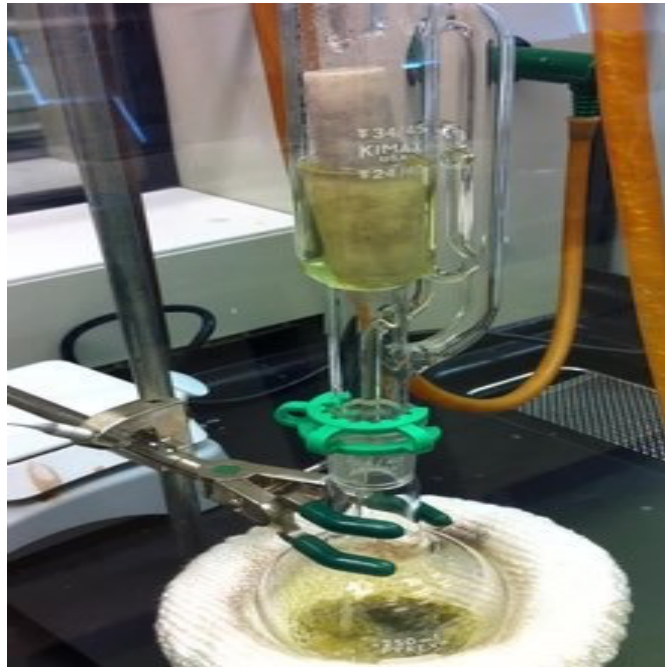
Figure 2.1: Soxhlet extraction of Aegle Marmelos
